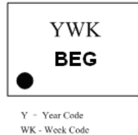
MSOP8/SOP8 Marking (Top View)
